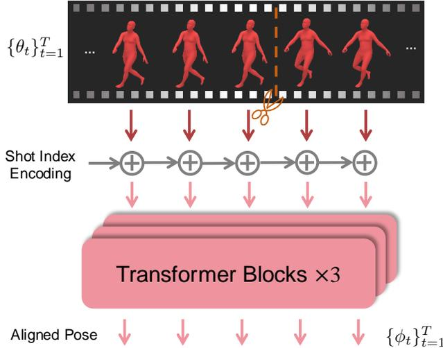
Figure 6. *ms-HMR* Structure. The initial human pose parameters  $\theta$  across multiple video shots are input into a transformer with shot-index-based positional encoding. This enables *ms-HMR* to generate consistent human poses across all shots in the video.
